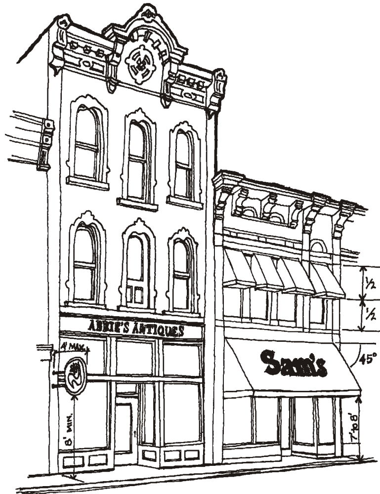
Diagram 2: Appropriate sign and awning locations and proportions. Note awning is between, not over, piers.
