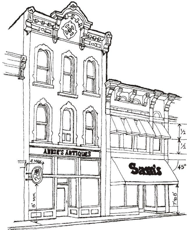
Diagram 1: Typical sign and awning locations and proportions. Note awning is between, not over, piers.
