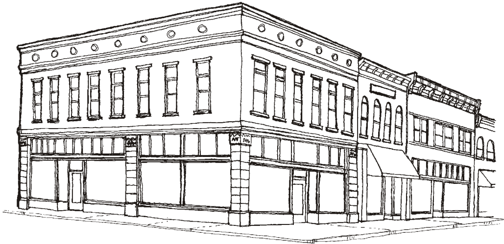
Diagram 1: Example of a corner infill building which exhibits similar characteristics to original buildings in same block, including alignment of storefronts, upper facade windows, and cornice.
